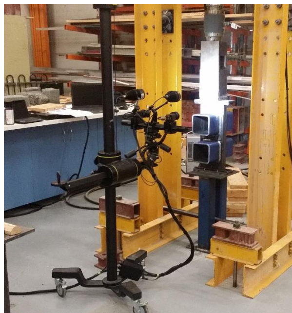
Figure 6. 10. Focusing the camera of the ARAMIS system to the target area around the first bolt, before applying the load on the specimen
