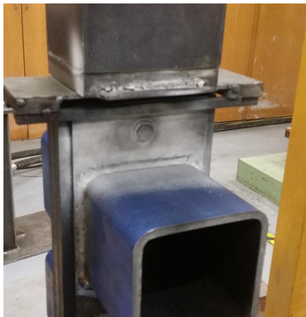
Figure 6. 9. The special paint applied around the area of the first bolt before focusing the camera of the ARAMIS system for strain measurements
