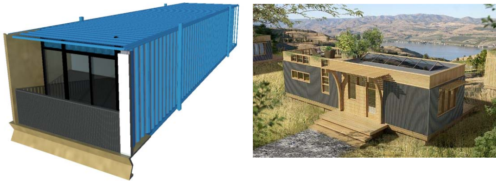
Figure 2. 1. A corner supported module (Left) and a Load Bearing Module (Right)
