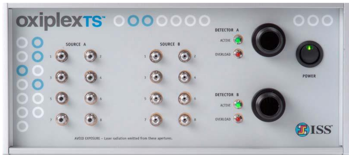
Figure 6-3 Front panel of the OxiplexTS™ (FD-NIRS) device.
