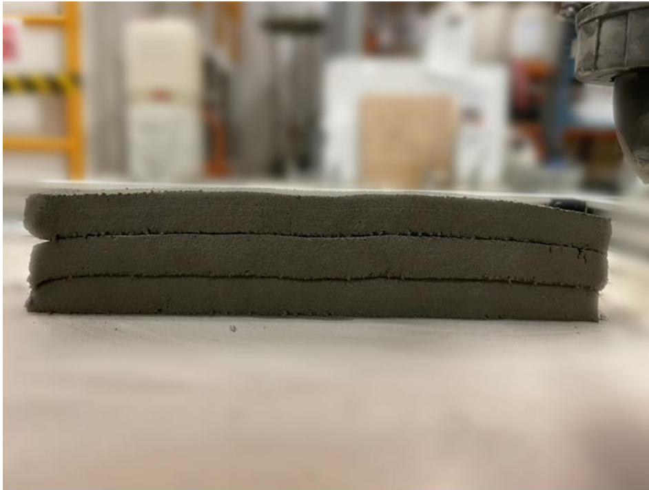
Figure S 2. Printing quality of three-layer specimen with S/C of 1.0.
