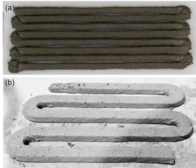
Figure 2.6. Suitable extrudability (no filament breakage or discontinuity) of (a) cement-based [21] and (b) FA-GGBS based [24] 3D printing concrete mixtures.
