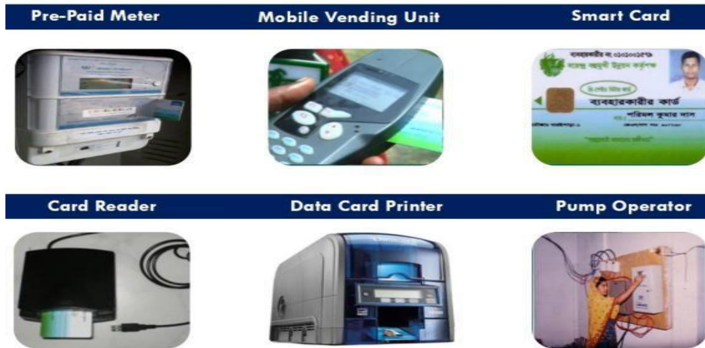
Figure 3 shows the components of a prepaid smart meter (source: Asaduz Zaman, ‘Participatory Irrigation Management: Barind Model a New Sustainable Initiative’ (2019) 7(6) Universal Journal of Management 220, 224).
