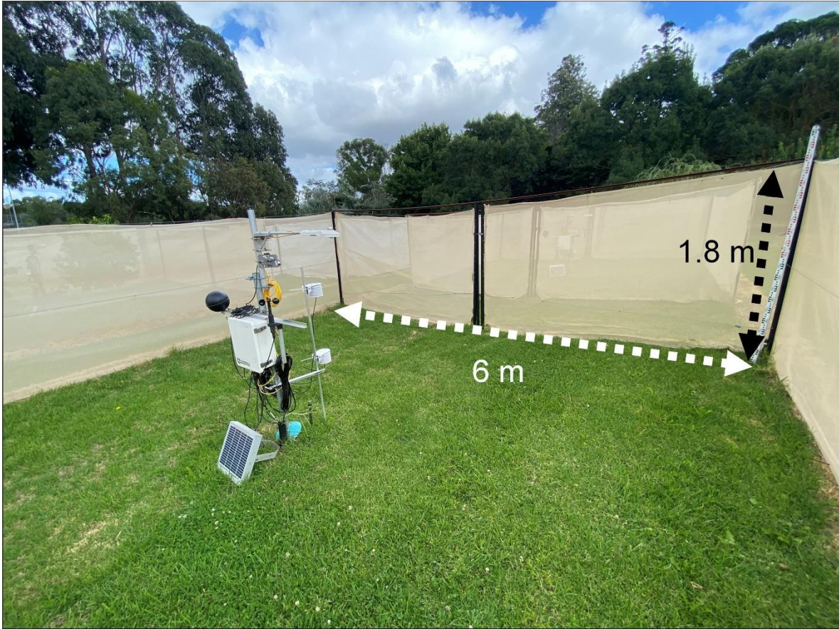
Fig. 6.1. Six identical plots (6×6 m) were set up at the Burnley Campus of the University of Melbourne. Three were unirrigated and three received 4 mm of irrigation at 13:00 every day. Each plot was surrounded by 1.8-m tall 70% shade cloth (SOLARSHADE™) and a climate station was installed at the centre of each plot to continuously monitor the microclimate, soil temperature and soil moisture content.
