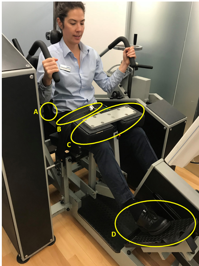
Figure 4 A participant seated on the MedX machine at 12° lumbar flexion. The MedX restraint system includes the pelvic restraint (A), lap belt (B), thigh restraint (C) and foot plate (D).
