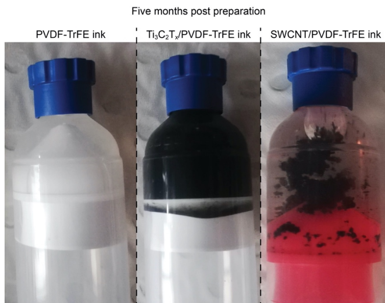
Figure 5.S3: Comparison of the stability of the PVDF-TrFE ink (left), \text{Ti}_3\text{C}_2\text{T}_x/\text{PVDF-TrFE} ink (middle) and SWCNT/PVDF-TrFE ink (right), five months after preparation of the ink.
