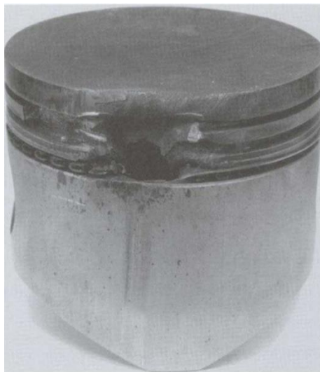
Figure 2-1 The damaged piston caused by knocking combustion [14].
