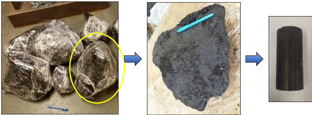
Figure 3-2 – Acquisition of coal samples as blocks and double sealed with polyethylene-films until the sample preparation to prevent the moisture loss during transportation and storage.
