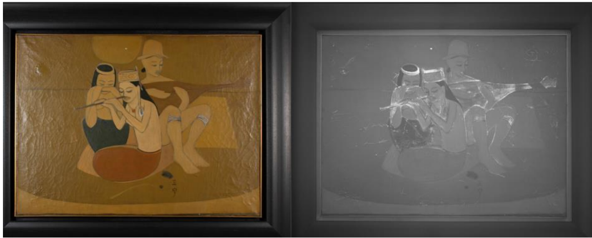
Figure 57a. Comparison images of visible light and transmitted-infrared photography showing less paint density around the figures and heavier paint in the background. Cheong Soo Pieng, Untitled (Three Figures, Musical Instruments) (1968).
