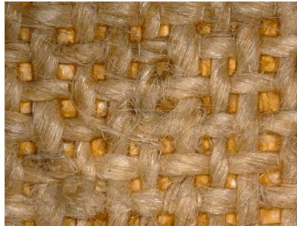
Figure 12. 50x Magnification of Holbein’s canvas fibres showing uneven threads and open weave. Georgette Chen, Satay Boy (1964).
