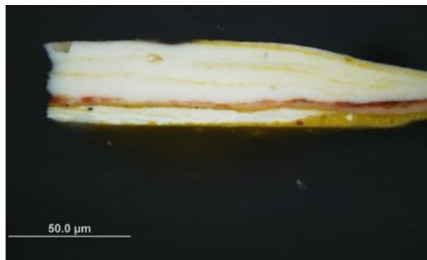
Figure 56c. 100x magnification detail of paint application technique featuring thin layers of paint observed in cross-section. Cheong Soo Pieng, Construction (1956).
