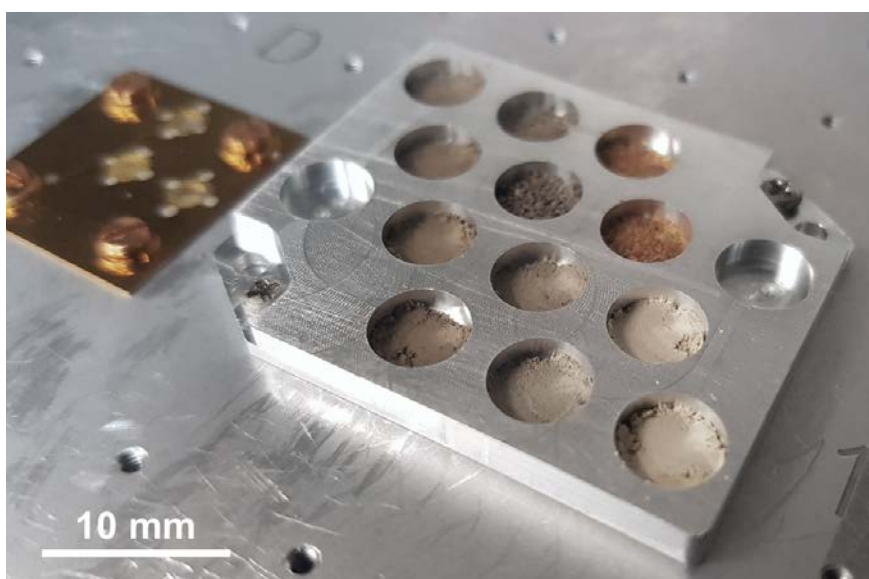
Figure 2 – Powder well plate mounted to the AXIS Nova ‘plain’ platen. Powder and particulate samples could be pressed into the wells, minimising cross-contamination of samples.
