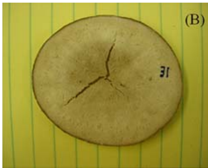
Figure 7.2.a: Internal cracking in freeze dried potatoes [1]
