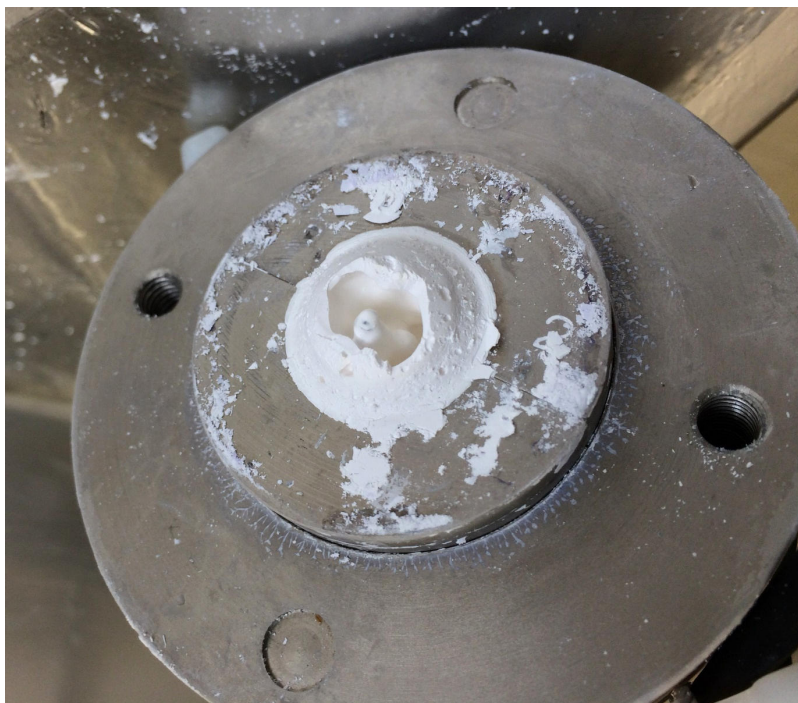
Figure 6.4.f: Failed suspension injection illustrating in-situ probe within sample injection chamber.
