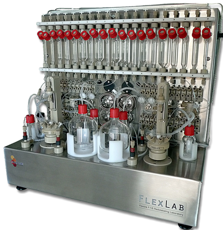
Figure 3-1: Iphase Flexlab for the automated synthesis of radiolabelled compounds
