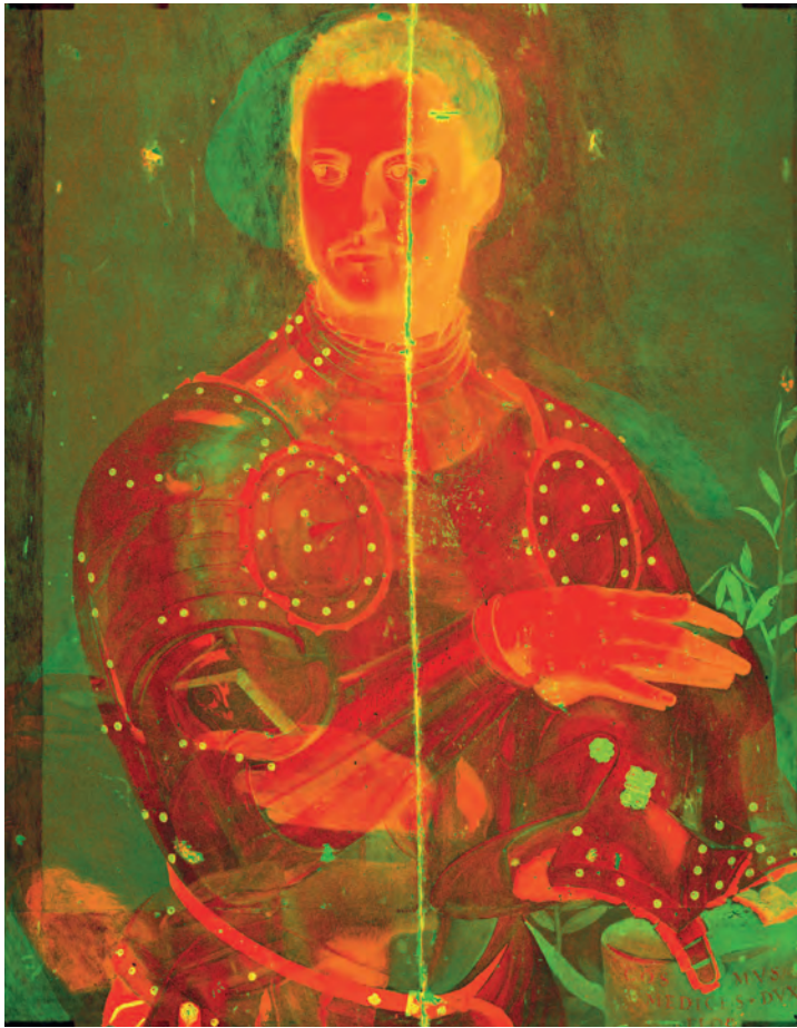
19. Composite XRF scan map of Fig.1 showing mercury (red) and iron (green). (© Art Gallery of New South Wales).
