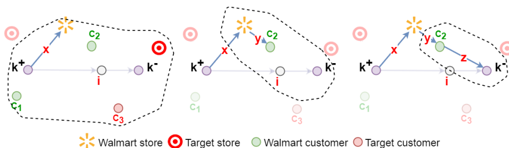
Figure 5.7: Left. An ellipse with threshold t is computed based on k^+ and k^- . Customers within it are not guaranteed to be visited after the driver visits Walmart. Center. In the next iteration, a new ellipse is computed with foci Walmart and k^- . The new threshold is t - x . Right. Ellipse has foci c_2 and k^- . Threshold is t - x - y . This is the last iteration.
