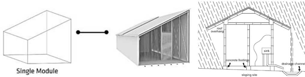
Figure 4: Single module proposed by Rodrigues and Henriques (2016) and design solutions proposed by Xiao and Paudel (2008).
