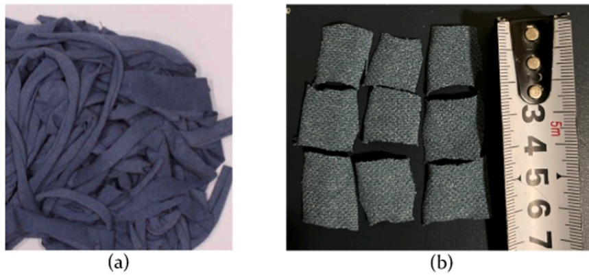
Fig. 1. (a) Waste fabric pieces from manufacturer; (b) Prepared waste fabric pieces 20 × 20 mm.
