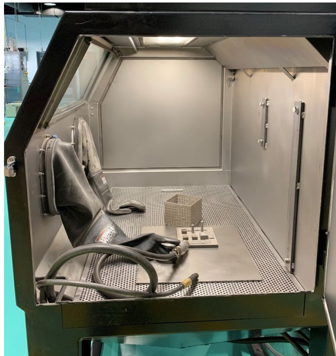
Figure 4.1: Inside view of powder recovery system (PRS).
