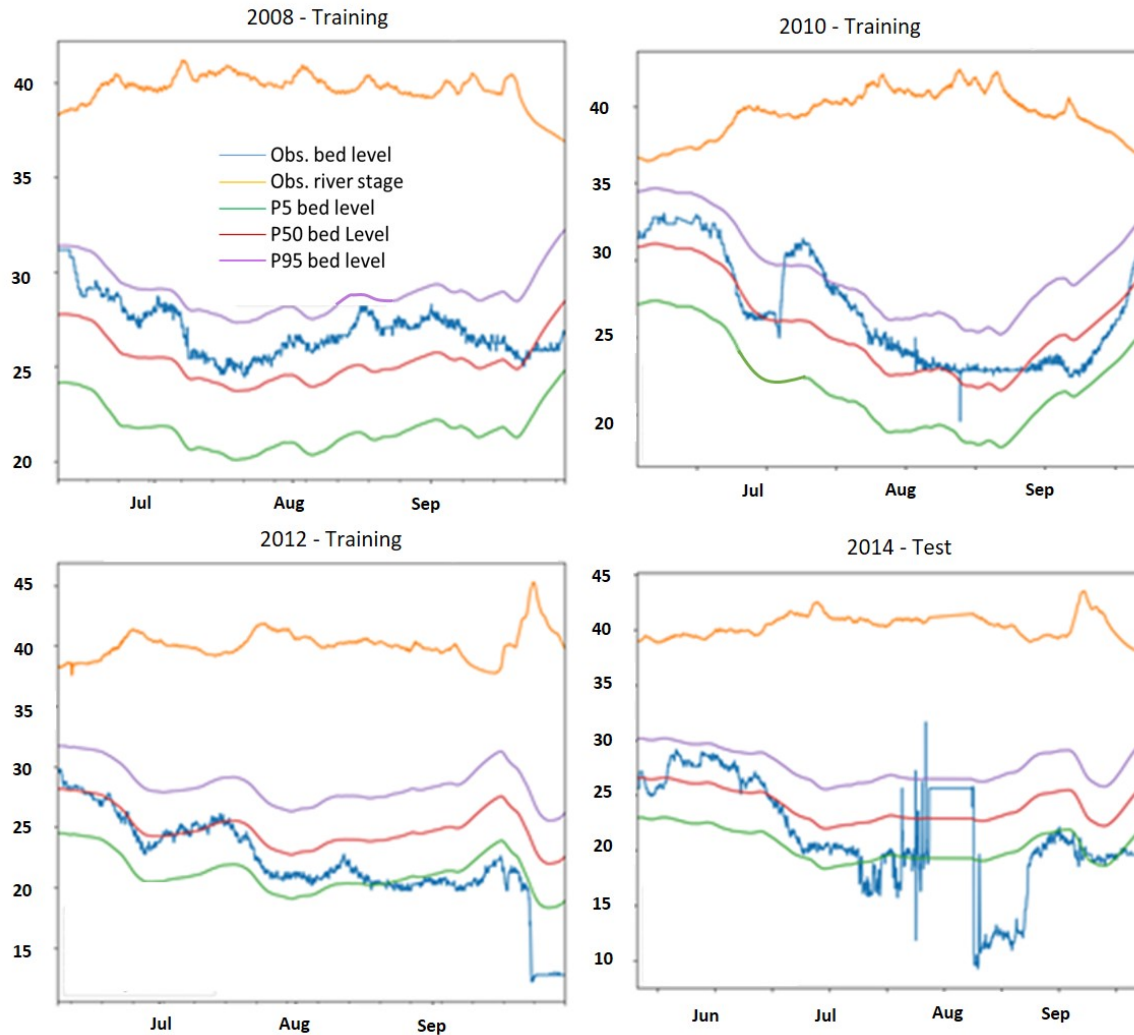
1 Figure 13 Model predictions on 2008-2012 training dataset and test dataset from 2014 (x axis is time, 2 y axis is elevation in ft).
