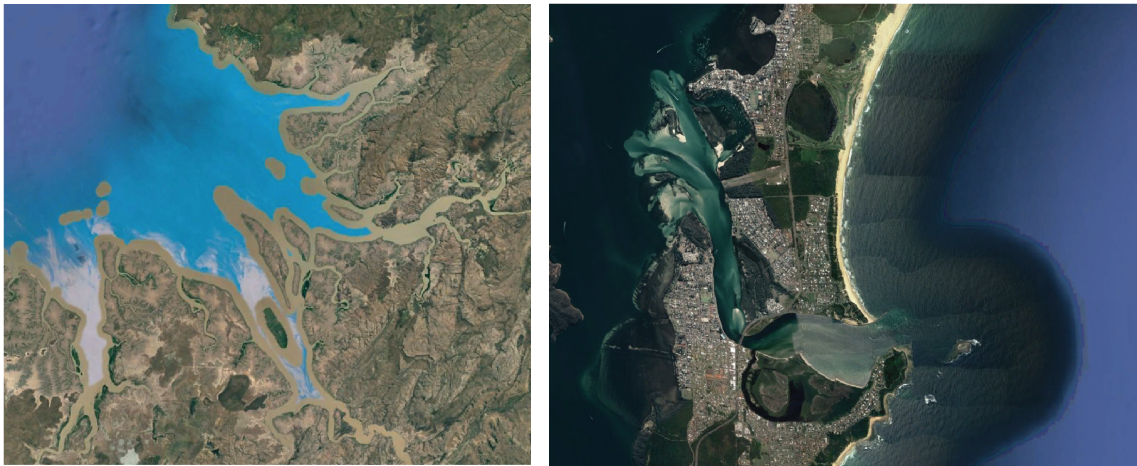
Figure 2.3: An example of typical shapes of tidal inlets - a tidal-dominated inlet in Victoria River, Northern Territory, Australia (left) and a wave-dominated inlet in Swansea, New South Wales, Australia (right). In the former, the mouth is larger because of the action of tides.
