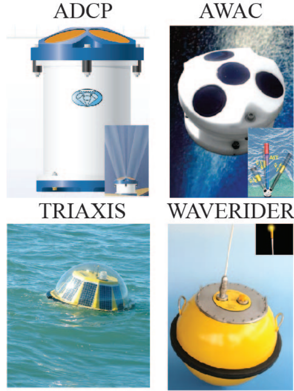
Figure 3.3: Several types of instruments used to measure waves and currents at PPH (AWAC, ADCP), SC (Waverider), and offshore (Triaxis).
