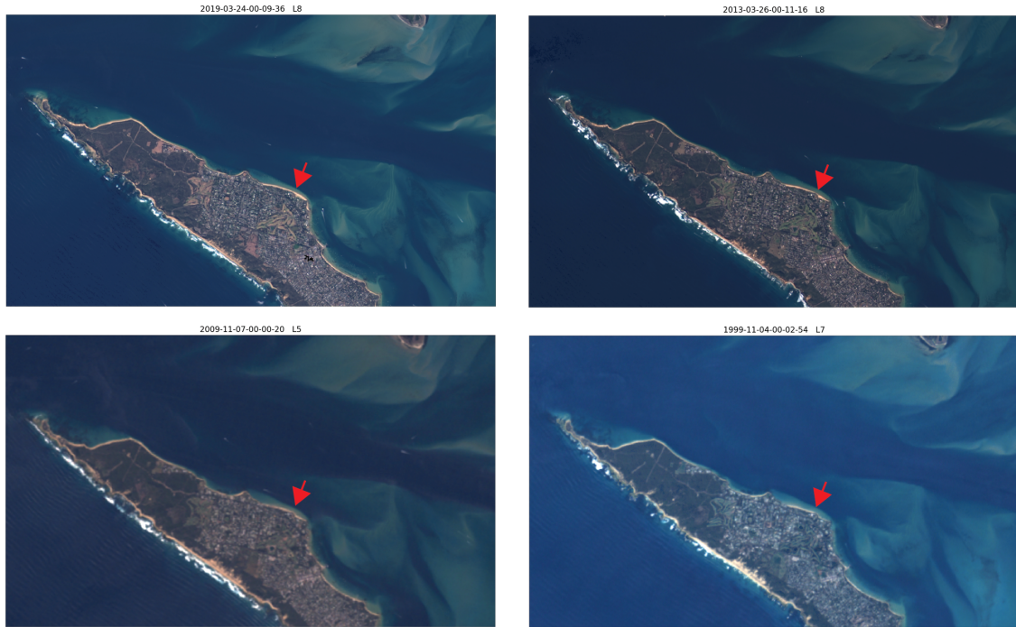
Figure 7.11: Changes in coastlines captured by Landsat 5, 7 and 8. The top panel (2019, 2013) is notably brighter in colour than the bottom panel (2009, 1999) in a region (red arrow) between Portsea and Sorrento, PPB.
