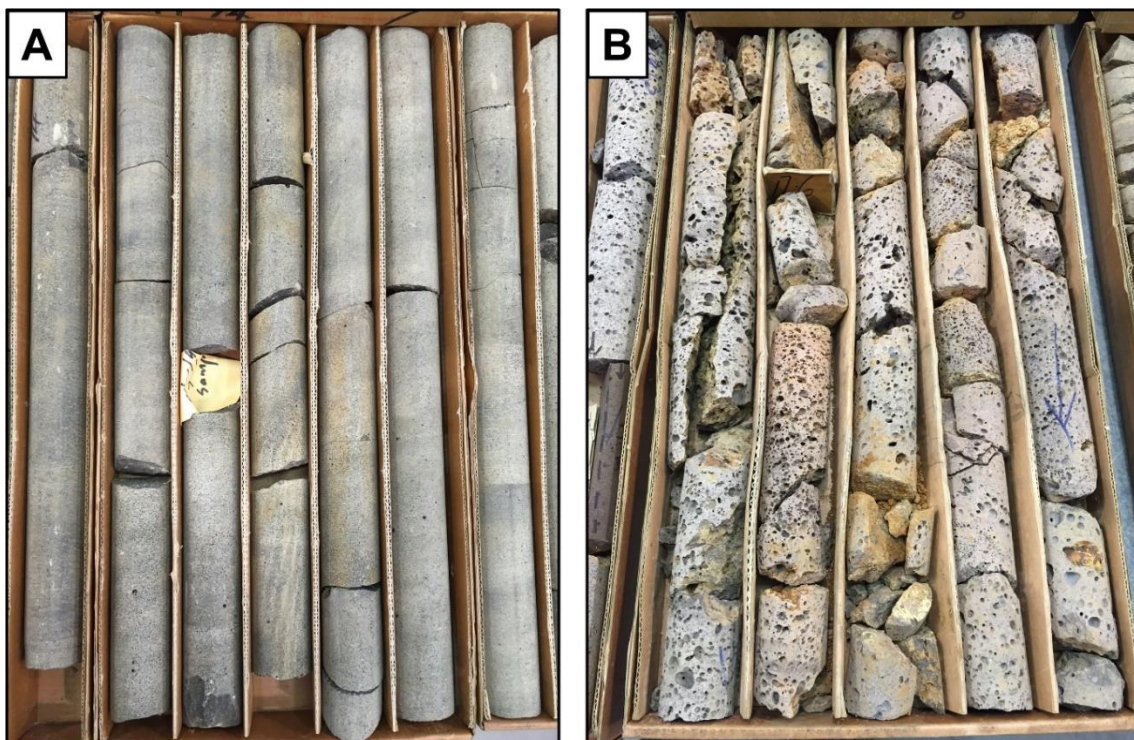
Figure 3.4: Borehole samples were preferentially selected from massive basalt in the middle sections of flows (a) , avoiding vesicular or altered sections (b) which were often at flow margins.
