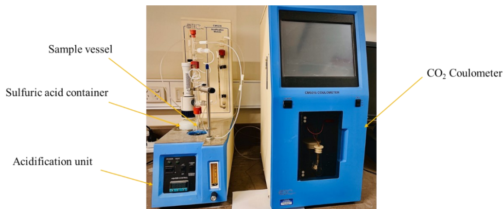
Fig. 3.3. Colourimetry titration equipment
