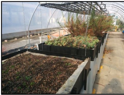
Fig. 1. Experimental set-up of 18 green roof modules under a polytunnel structure equipped with an overhead rainfall simulator.
