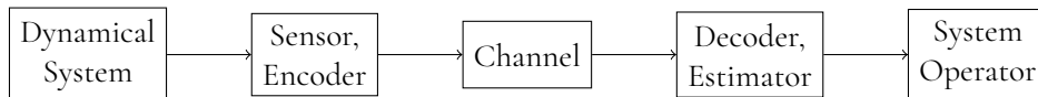
Figure 1.2: Illustrative model of the state estimation problem over point-to-point noiseless communication channel.
