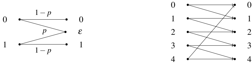
Figure 2.5: Channel transition diagram of (a) Binary Erasure Channel with C_0 = 0 ; (b) Pentagon Channel with C_0 > 0 .
