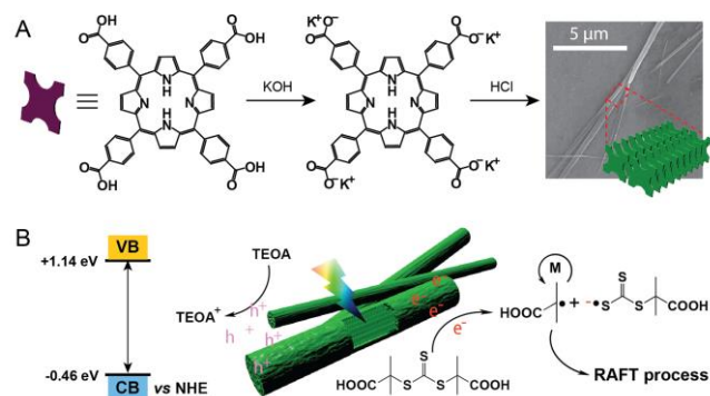
Scheme 1. (A) The synthetic strategy for rod-like SA-TCPP and (B) schematic mechanism of the photocatalytic PET-RAFT polymerizations by SA-TCPP.
