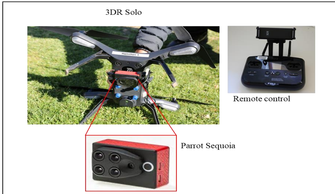
Figure 3 An aerial platform (3DR Solo) equipped with a Parrot Sequoia multispectral camera on board for HTP of perennial ryegrass plants deployed in Agriculture Victoria Research, Hamilton Centre, Australia.
