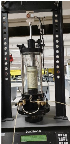
(c) Sample during the CD test
