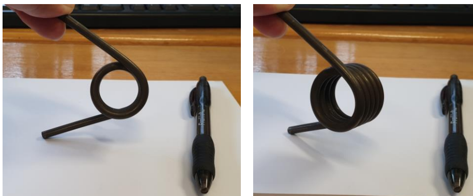
Figure 4-34 Fabricated mild spring rotational spring, with 171 N-mm/deg rotational stiffness.
