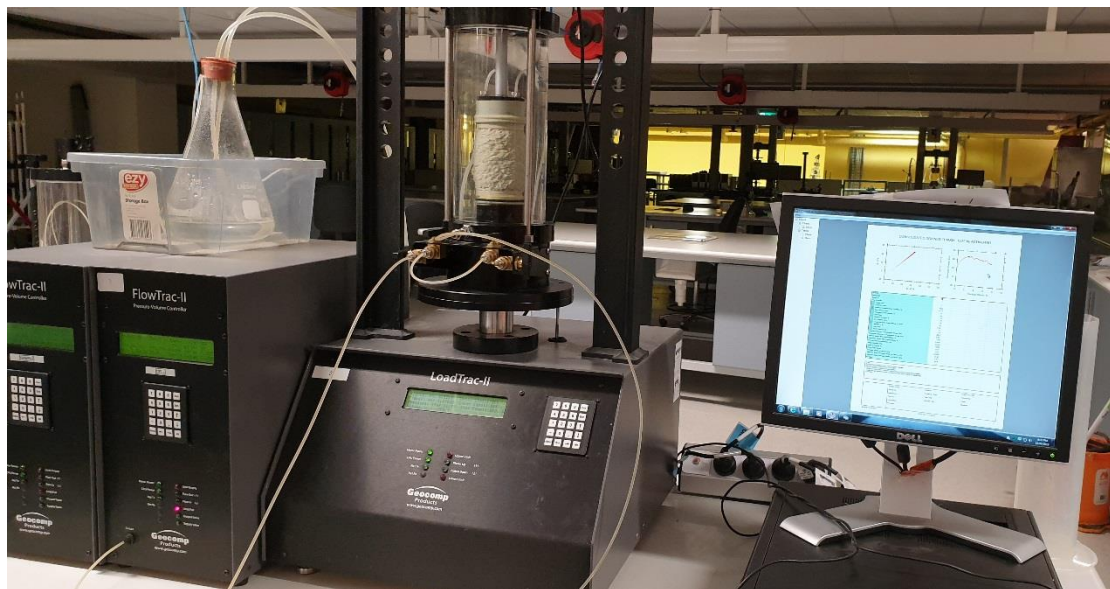
Figure 5-3 Triaxial test set up for the CD test on the crushed rock.
