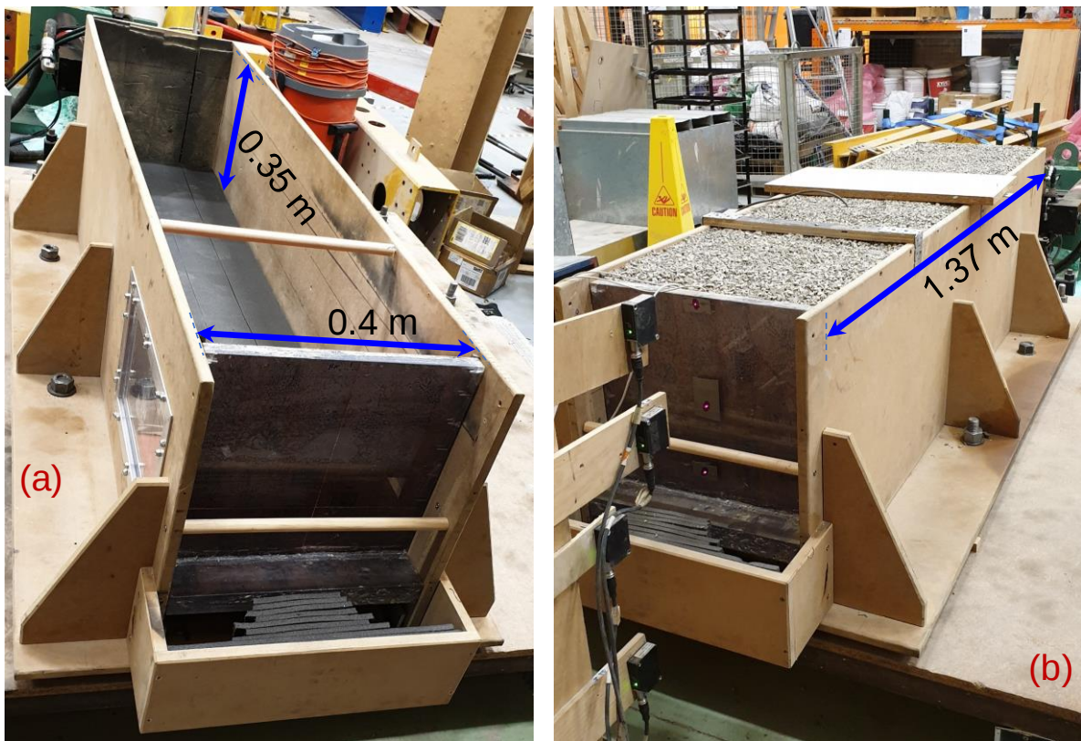
Figure 4-38 (a) High density foam applied at scaled down model base and backside (left), (b) constructed scaled down RW model supported by rotational springs.
