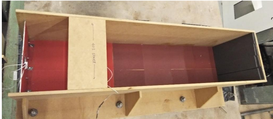
(b) Sandpaper placed at wooden container base.
