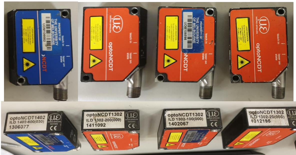
Figure 4-5 Laser transducer used for capturing displacement response of scaled down RW model.
