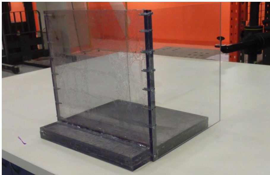
Figure 3-6 Scaled down RW model, fabricated using Polycarbonate sheets.
