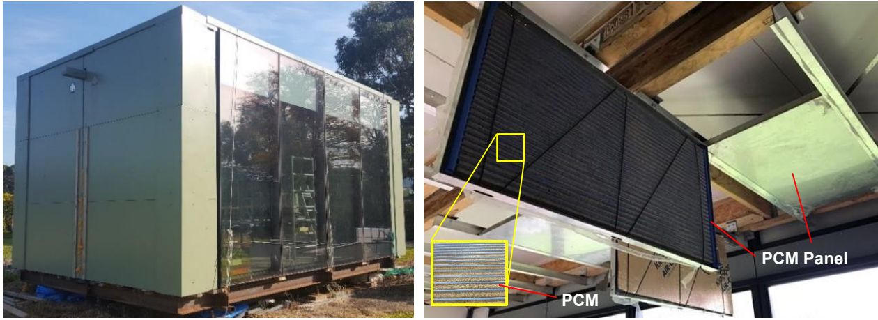
Fig. 1 The test cabin at the University of Melbourne (left), and PCM ceiling panels with capillary tubes (right)
