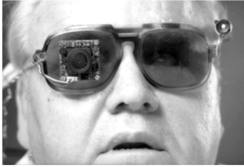
(a) Images of glasses-mounted camera worn by a patient implanted with the Dobelle cortical prosthesis (Image adapted from Dobelle, 2000)
