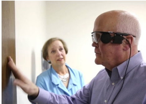
(c) Images of glasses-mounted camera and wireless transmitter worn by a patient implanted with Second Sight's Argus II. (image adapted from de Cruz et al, 2016)
