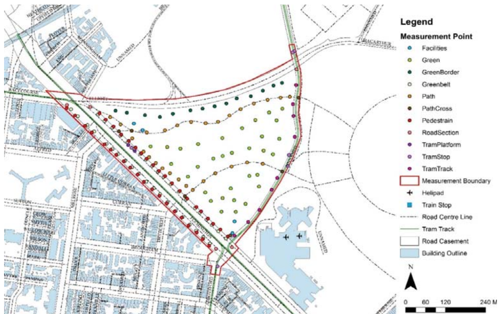
Fig. 2: Designated noise measuring points on the site
