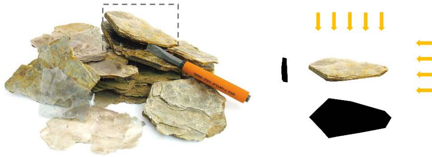
Figure 2.1. 2D particle shape is subject to the projection, especially for platy grains such as mica (Teachers 2012).
