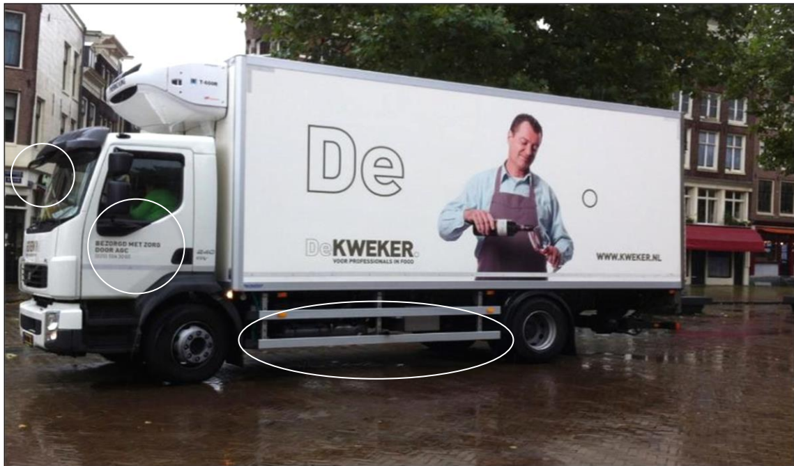
Figure 5-5 Truck with improved vision, mirrors, and side under-run
